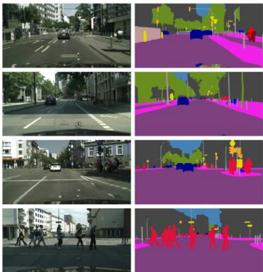
Figure 6.3: Semantic segmentation results with the Pyramid Scene Parsing Network [Zhao et al., 2016].
